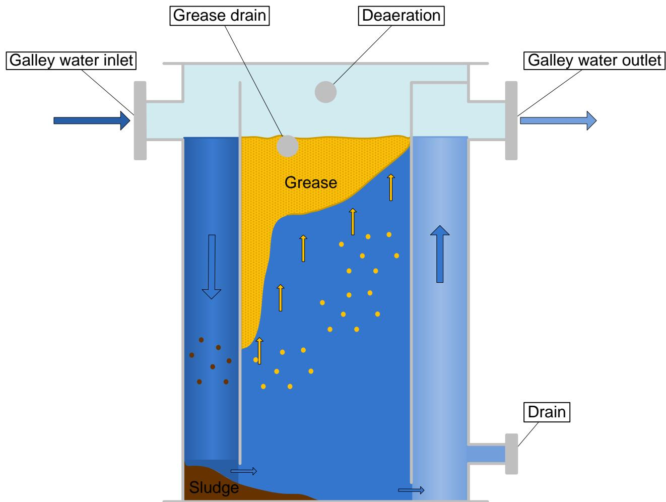
A grease trap removes fat, oil and grease (called FOG) and solids (food particles, sand and grit etc.) by a gravity separation process.
