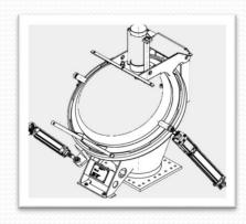
Feed hopper with 130l volume as part of the pressure vessel. Opens and closes automated. Pneumatic seals ensure safe operation.
