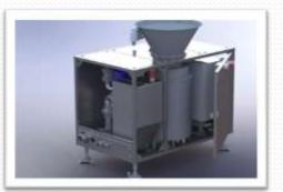
Cabinet holds controls. electrical installation, vacuum buffer tank, valves and food waste disposer (optional).
