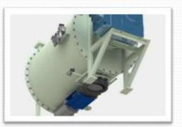
Double walled tank to circulate cool water to cool down bio waste before discharging it into incinerator.
