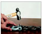
Place the coupler link on its side and using a hammer, drive the locking pin into the clevis ear until it is flush with the outside surface.
