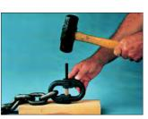
Drive the pin through the assembled link ends and sleeve until the end of the pin is flush with the outside of the connecting link halves.
