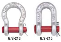
Round Pin Shackles can be used in tie down, towing, suspension or lifting applications where the load is strictly applied in-line. Round pin shackles should never be used in rigging applications to gather multiple sling legs, or where side loading conditions may occur.
