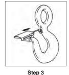
3. Position latch to side of hook points. Slide latch onto spring legs between lockplate and latch body until latch is partially over hook cam. Then depress latch and spring until latch clears point of hook.
