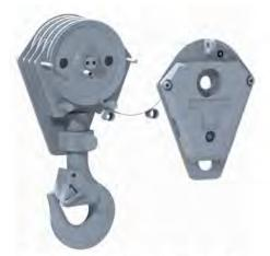
Minimized height, for maximum headroom. Traditional guards/guides facilitate reeving without a fitting.
