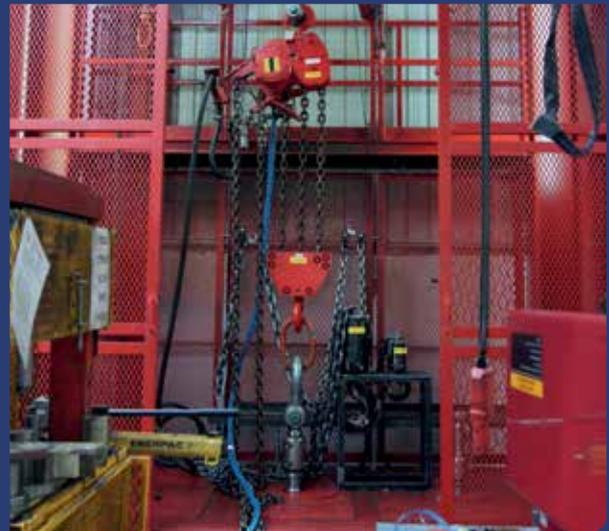
In our professional workshop we have a fully equipped dynamic test rig. This test rig is calibrated and certified according the European standard NEN - EN 818.
